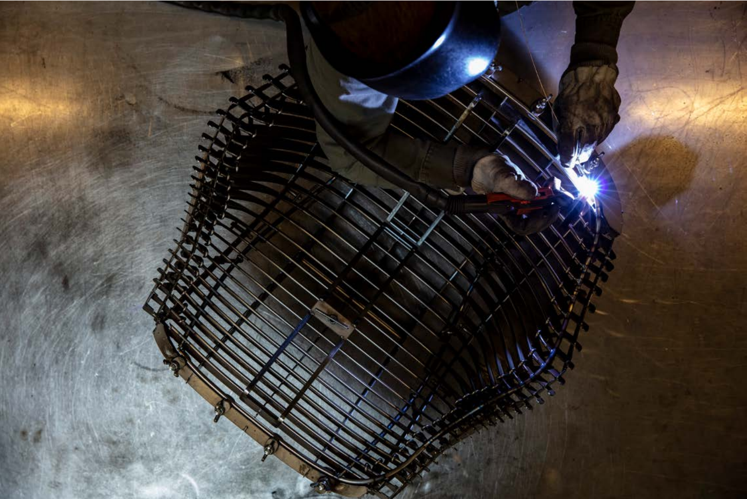
This spread Welding by hand - it takes 268 welds to make a single Wire Dining Chair steel seat
